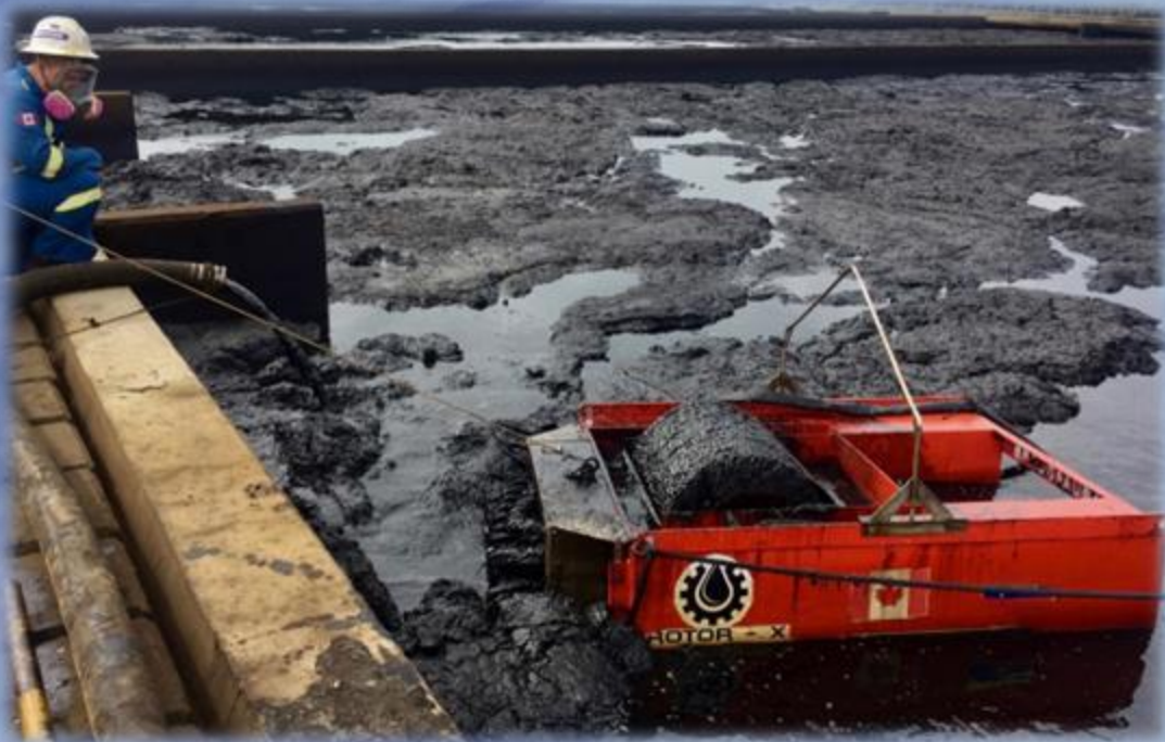
RBS TRITON™ 60 oil skimmers – Chevron Refinery
